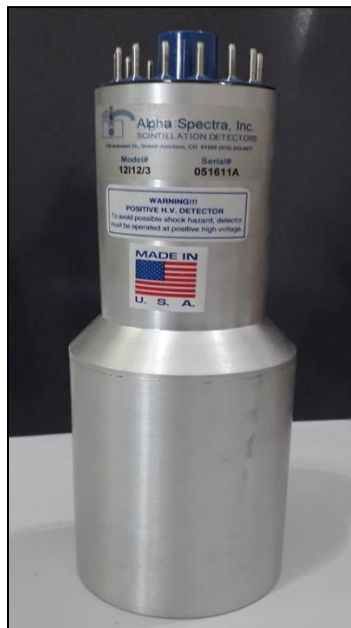
Fig. 1 – Sodium Iodide scintillator and photomultiplier used in this gamma radiation measurements (Aware Electronics, INC, USA) [9].
