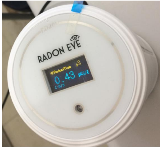
Fig 2 – Top view of RD200 Radon Eye ionization chamber used for monitoring radon gas [10]
